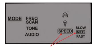
When SPEED icon is highlighted, use the Plus / Minus Menu buttons to select desired coil swing speed.
