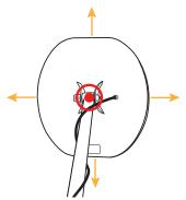
For very small, shallow targets, use either front corner of the mono coil to more precisely locate the target.
