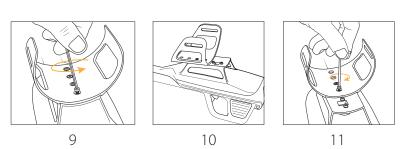
Caution: Always power OFF your Axiom before changing searchcoils. Disconnecting and reconnecting coils while the detector is powered on could damage the searchcoil and/or the detector's electronics.
